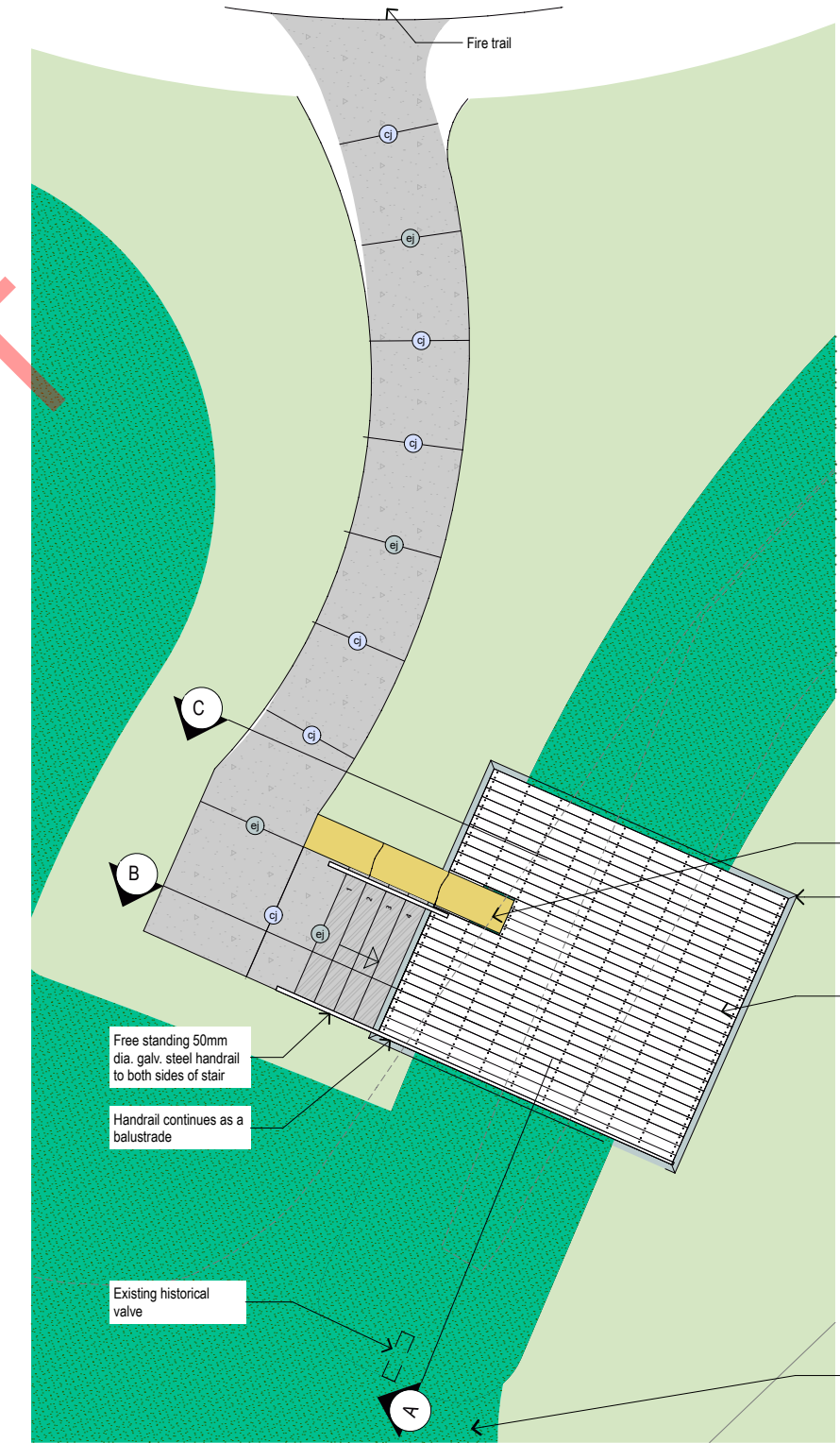
D VALVE VIEWING PLATFORM STRUCTURE PLAN
